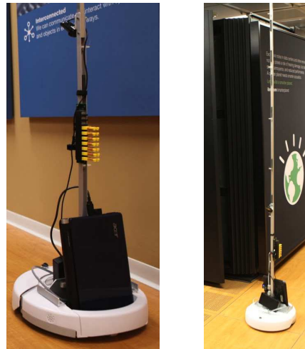
Fig. 1. The data center mapping and monitoring robot.
