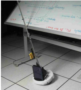
Figure 5: The robot getting upended while scooting under a mobile whiteboard in the data center.
